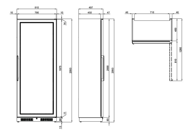
ELECTRICITY SUPPLY: 230V ~ 1 – 50Hz Wire lenght 1,5mt (\*SCHUKO plug)
